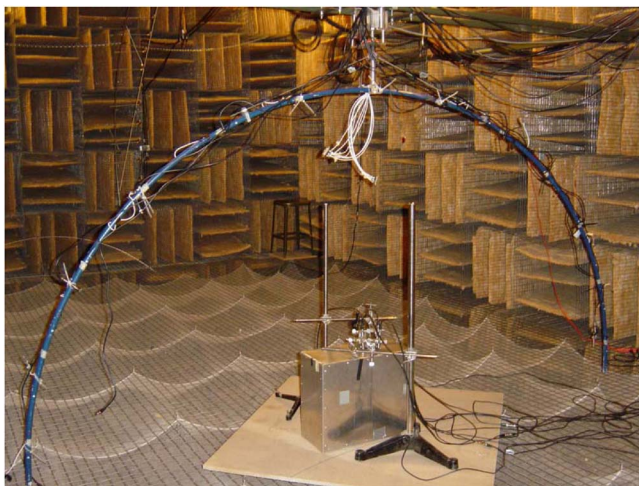
Fig. 6—An aluminum mock computer casing shown under a rotating semicircular microphone boom located in the anechoic chamber on the Brigham Young University campus.
